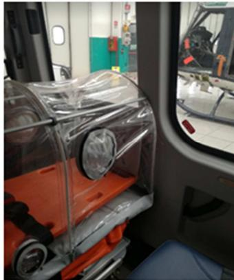
Results of tests performed during the initial installation have shown that an adequate flow rate thorough the HEPA filter is ensured when at least two rows of filter holes are left free with a sufficient clearance ( 3-4 cm ), this can be easily achieved by taking advantage of the recess existing in correspondence of the emergency exit as shown by the arrow in the figure below
