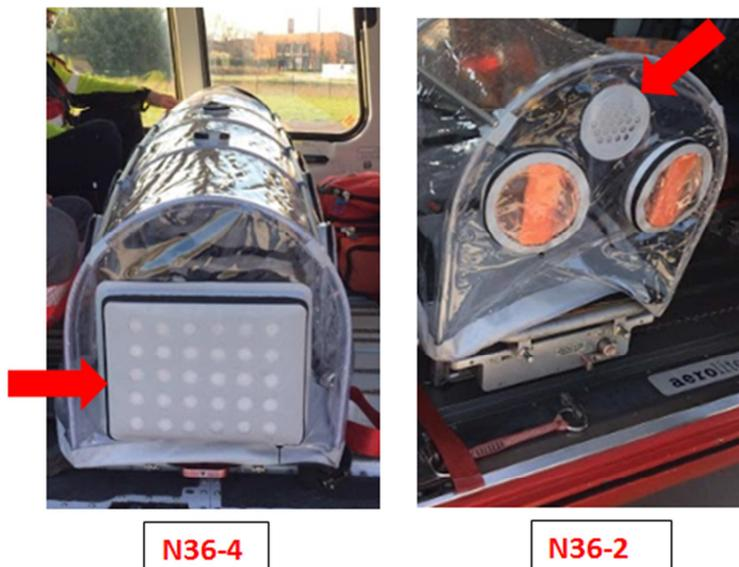
Should the HEPA filter completely rests against the door as shown in the figure below, a risks exists that the air flow rate thorough it may be reduced with obvious danger for the patient inside.
