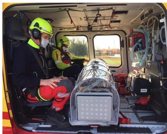
In this way the straps, securing the patient to the system and the system to the Aerolite stretcher can react the forward accelerations experienced in case of emergency landing.
