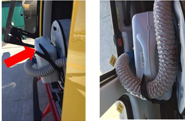
As a result of this operation, the overall length of the N-36 system is reduced and this can limit the maximum height of the patient who can be boarded .
