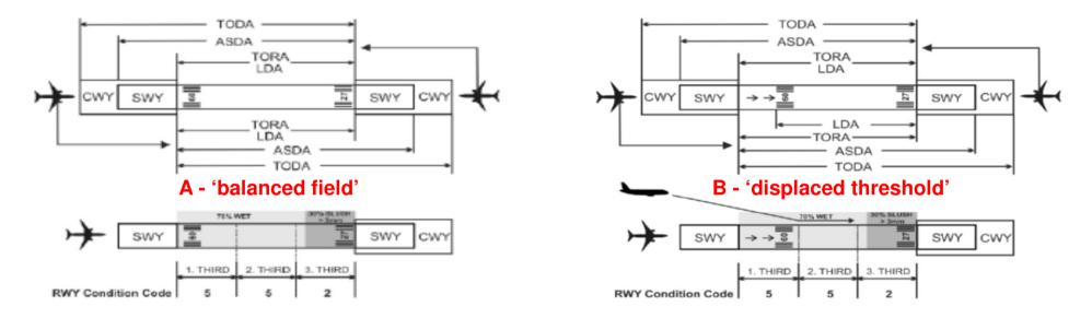
This is an important concept for flight crew to understand, especially when landing on a runway with a <u>significantly displaced</u> threshold, performing an intersection take-off, or part of a runway is declared as a RESA but still available for take-off.
