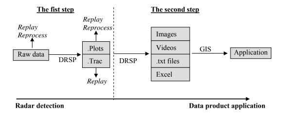
Figure 6-2. Flowchart of Radar Data Processing
