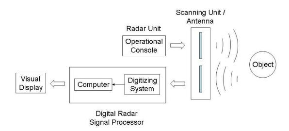
Figure 2-1. Basic Radar System Components
